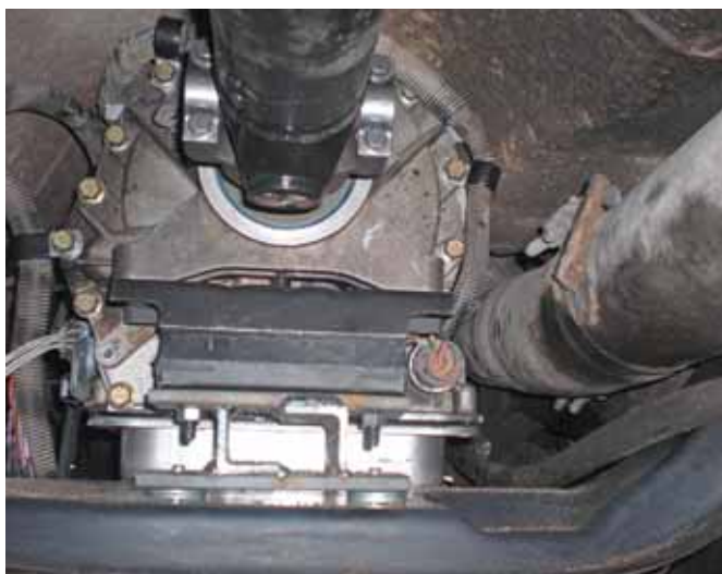
Even with a 5-inch exhaust system, there's room for the Allison unit, as this view from the rear shows.
