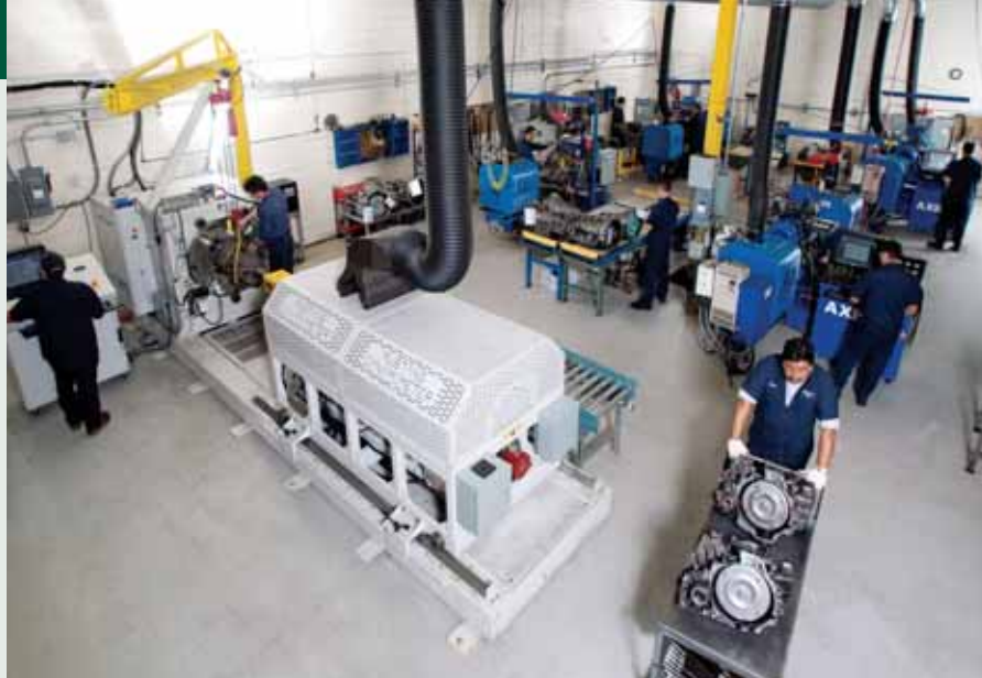
Each of the five dynamometers has been specifically enhanced to perform certain tests required by the ETE production team.
