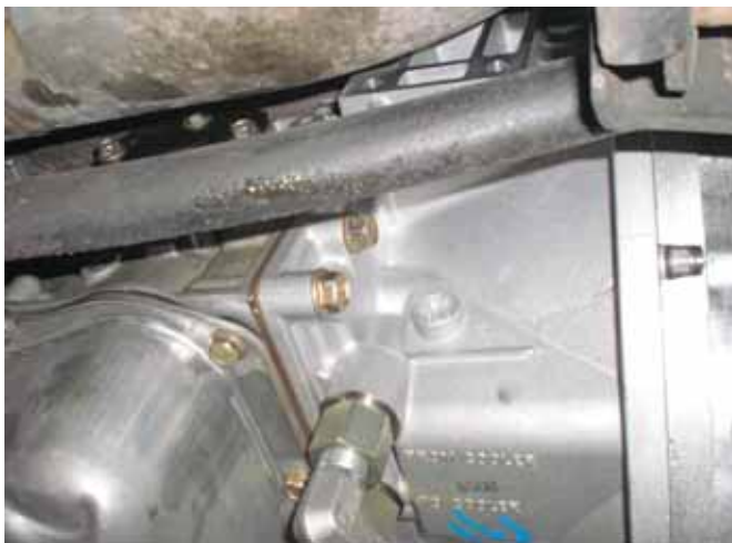
One of the Allison's 5/8-inch cooler-line fittings
