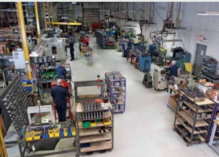
The ETE machine shop splits its time between remachining parts and creating specialized tooling and fixtures for the plant.
