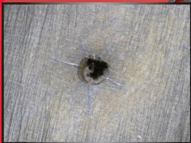
The 2-3 Accumulator Piston Spring Retainer Can Damage Stock Plates
