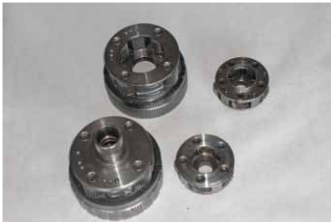
Note the difference in size between the Allison and 47RE planetaries.
