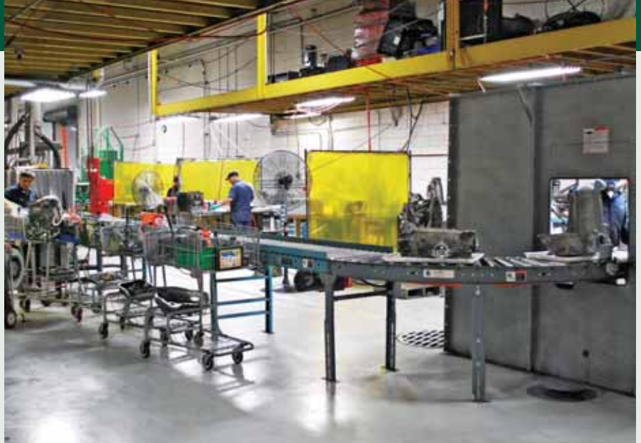
A conveyor moves cores through the disassembly, cleaning, paint and case prep processes.
